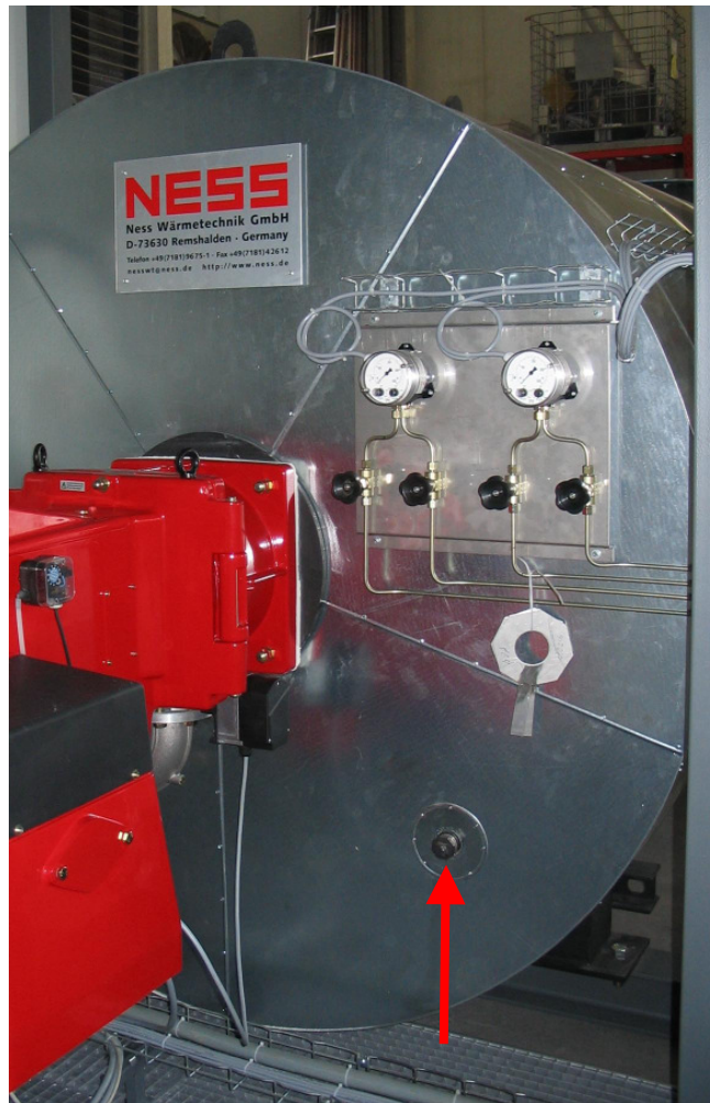
Picture 2: Each Ness heater comes with a fire extinguishing nozzle.
