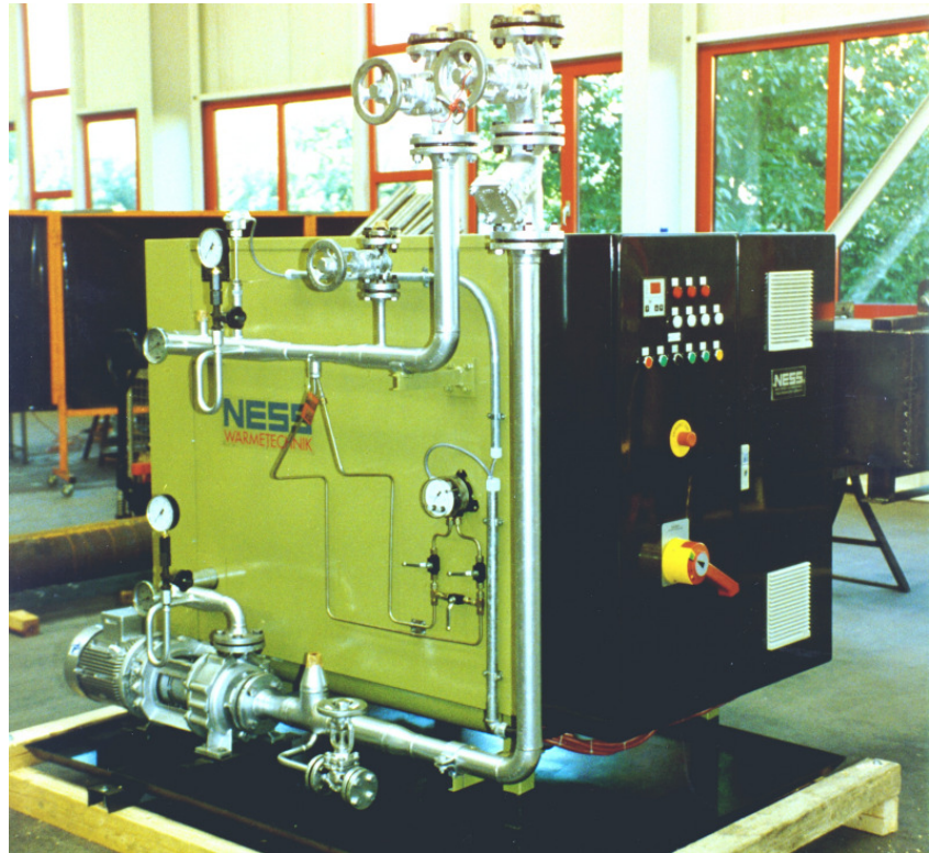
Picture 2: Ness electrical thermal oil heater EWE 270 (270 kW)
