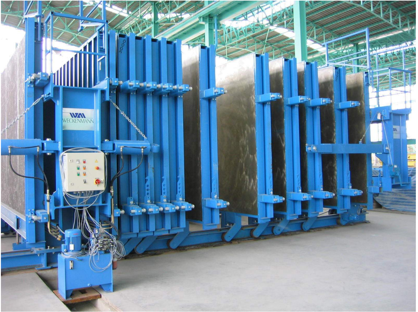
Picture 2: Thermal oil heated battery mould for concrete wall panels (picture by courtesy of Weckenmann Anlagentechnik GmbH & Co. KG)
